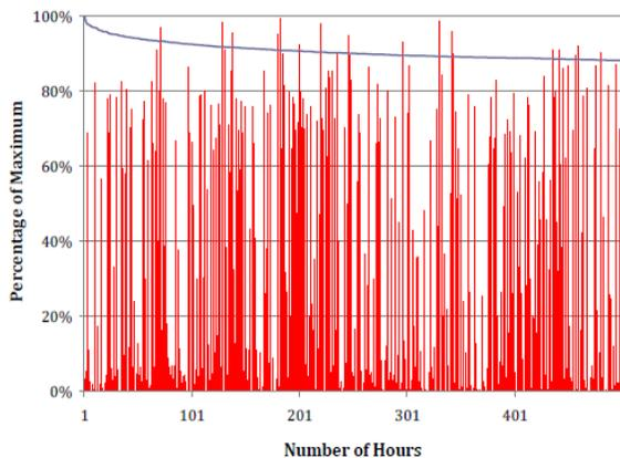
**FIGURE 3: THE POOR CORRELATION OF WIND OUTPUT WITH SYSTEM LOAD IS ILLUSTRATED BY THIS CHART, WHICH SHOWS FRACTIONAL WIND OUTPUT (RED LINE) IN THE 500 HIGHEST-LOAD HOURS OF 2009 (BLUE LINE).**
